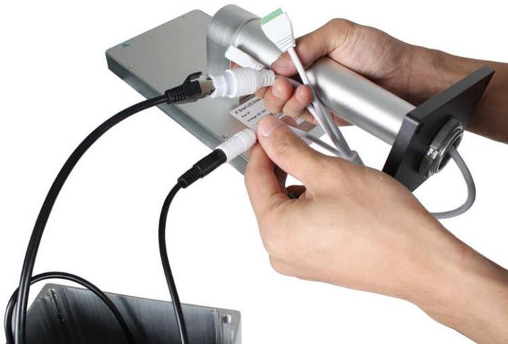
Connect the Ethernet and power ports from the display unit to the corresponding cables from the pole. Disregard the two cables with green ends, they are not needed immediately and are used only for Wiegand and Relay interfaces.
