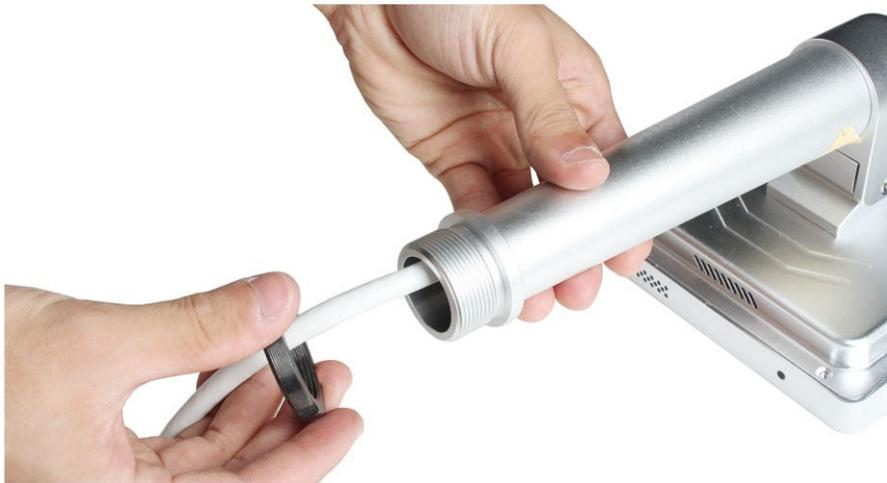
Remove the connector ring from the neck of the display unit. The end of the cable has 4 connectors; take them out through the ring one by one.
