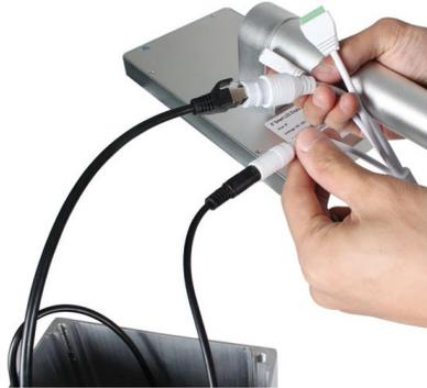
Connect the Ethernet and power ports from the display unit to the corresponding cables from the base unit. Disregard the two cables with green ends, they are not needed immediately and are used only for Wiegand and Relay interfaces.
